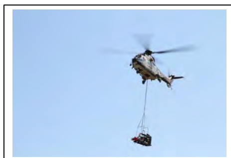
Figure 6: Air transportation of mobile equipment during an emergency drill exercise.
