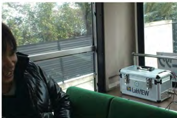
Figure 2: In-vehicle unit of KURAMA-II. All components are placed in a small tool box for a better handling. The in-vehicle unit of KURAMA-II is usually placed in the backside space of the rear seat row, corresponding to the center site of the road.
